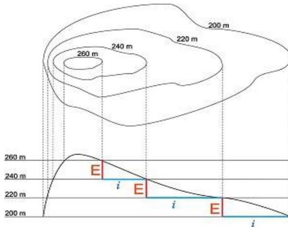
On a map, you are looking straight down, so it is difficult to see the change in elevation of the ground. As you can see in this image, a topographic map uses lines to determine the heights of features such as mountains and valleys. Topographic maps can show the heights of features a variety of ways, including contour lines, relief, and colour.
